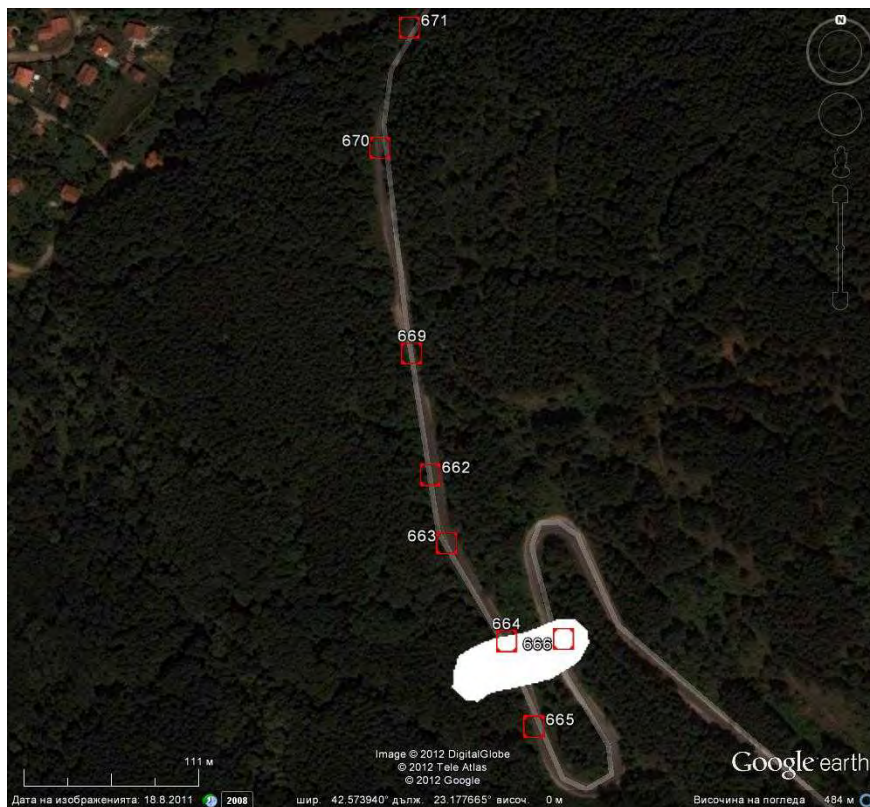
Figure 2.2. Location of landslide along the road Rudartsi-Kladnitsa and possible unstable sites
