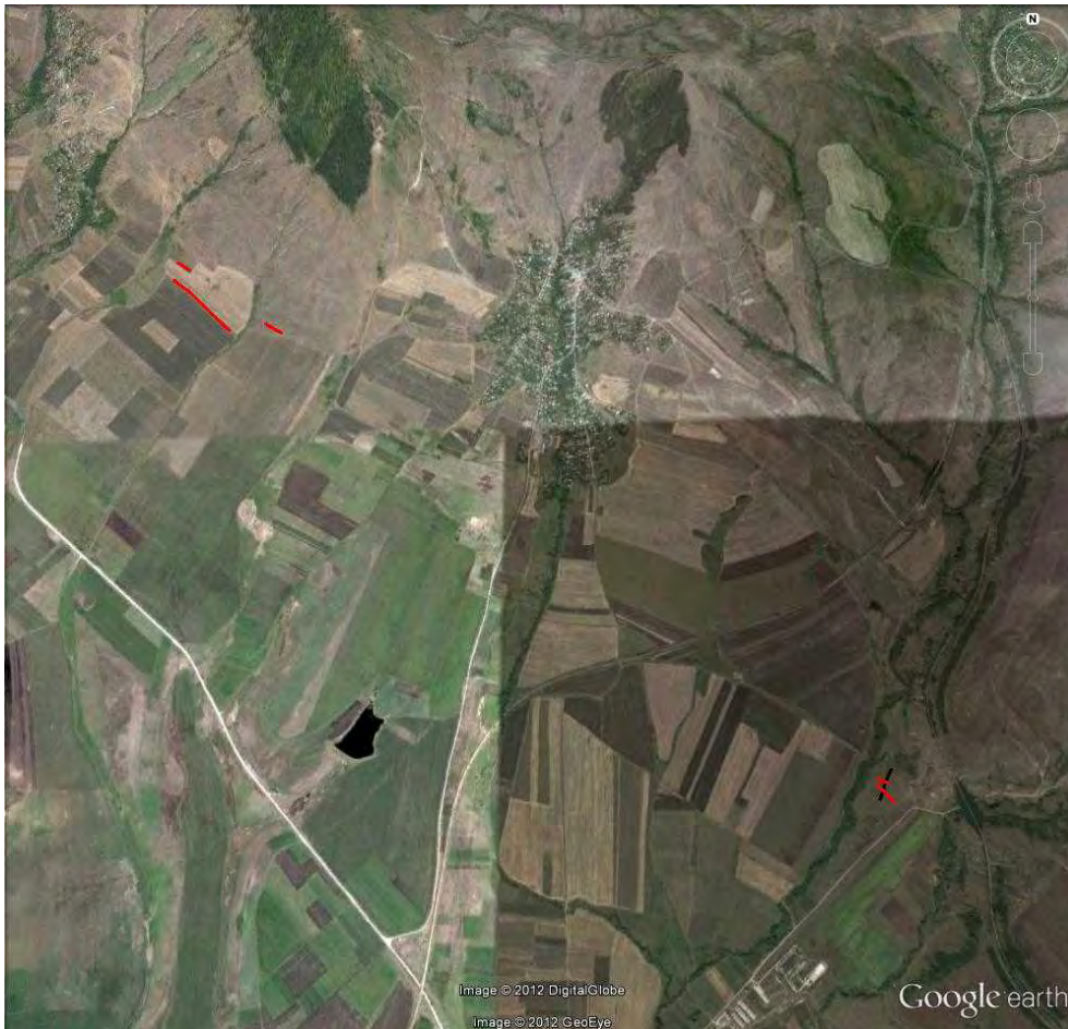
Figure 3. Map of observed coseismic geological effects. Red lines show position of ground cracks. Black line: position of the resistivity profile.
