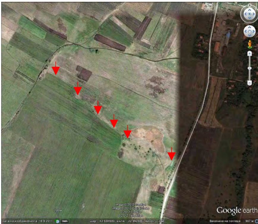
Figure 2.6. Satellite image of the gentle landslide and the visible fault trace (red arrows)
